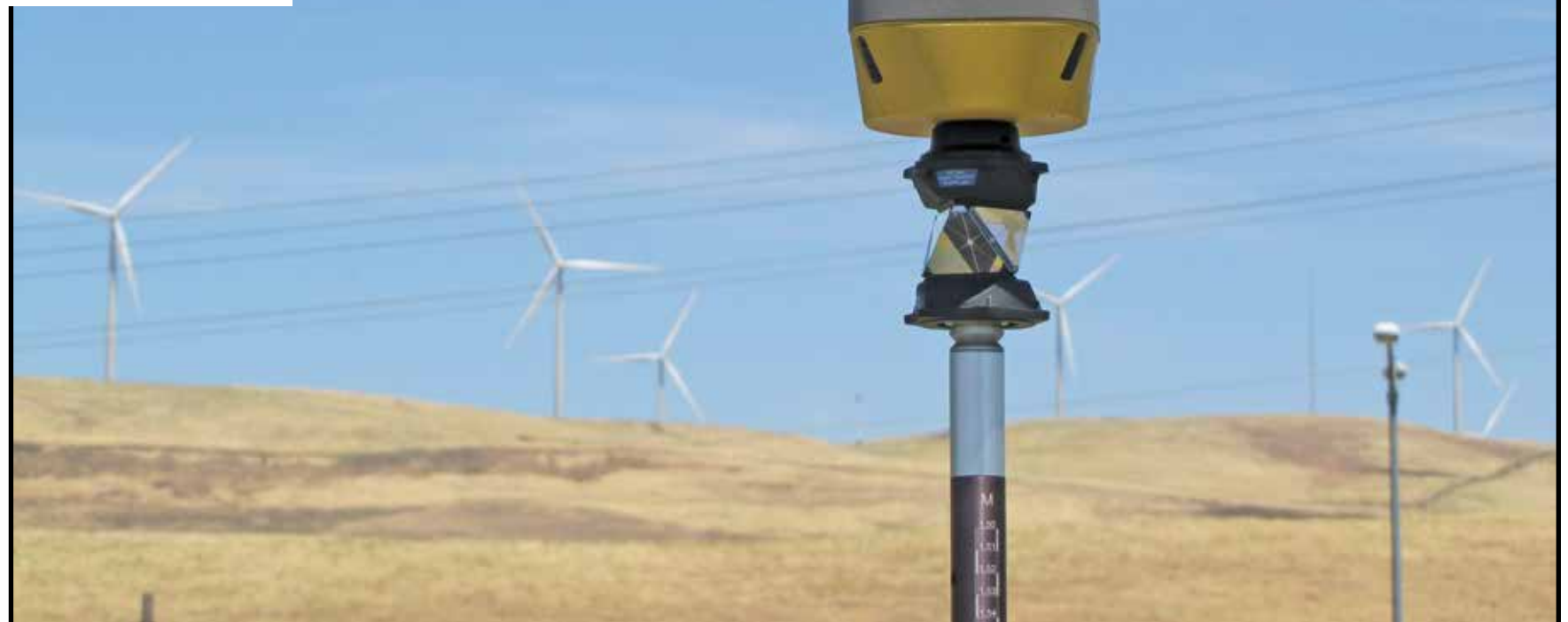
The "HR" in the HiPer HR stands for hybrid rover, Topcon's new integrated GNSS plus IMU platform designed to accommodate additional development.
